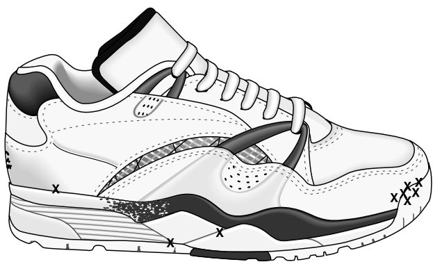
Figure 8.7. Defect location check sheet lamination complaints.
